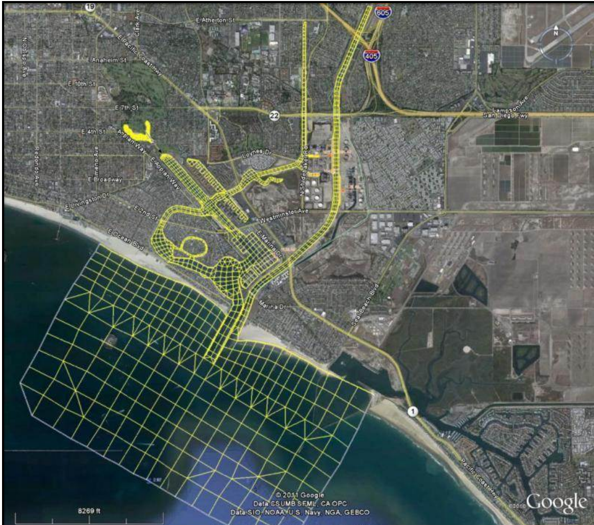
Figure 3-1. Finite Element Model for the Los Cerritos Wetlands (aerial image courtesy of Google Earth)
