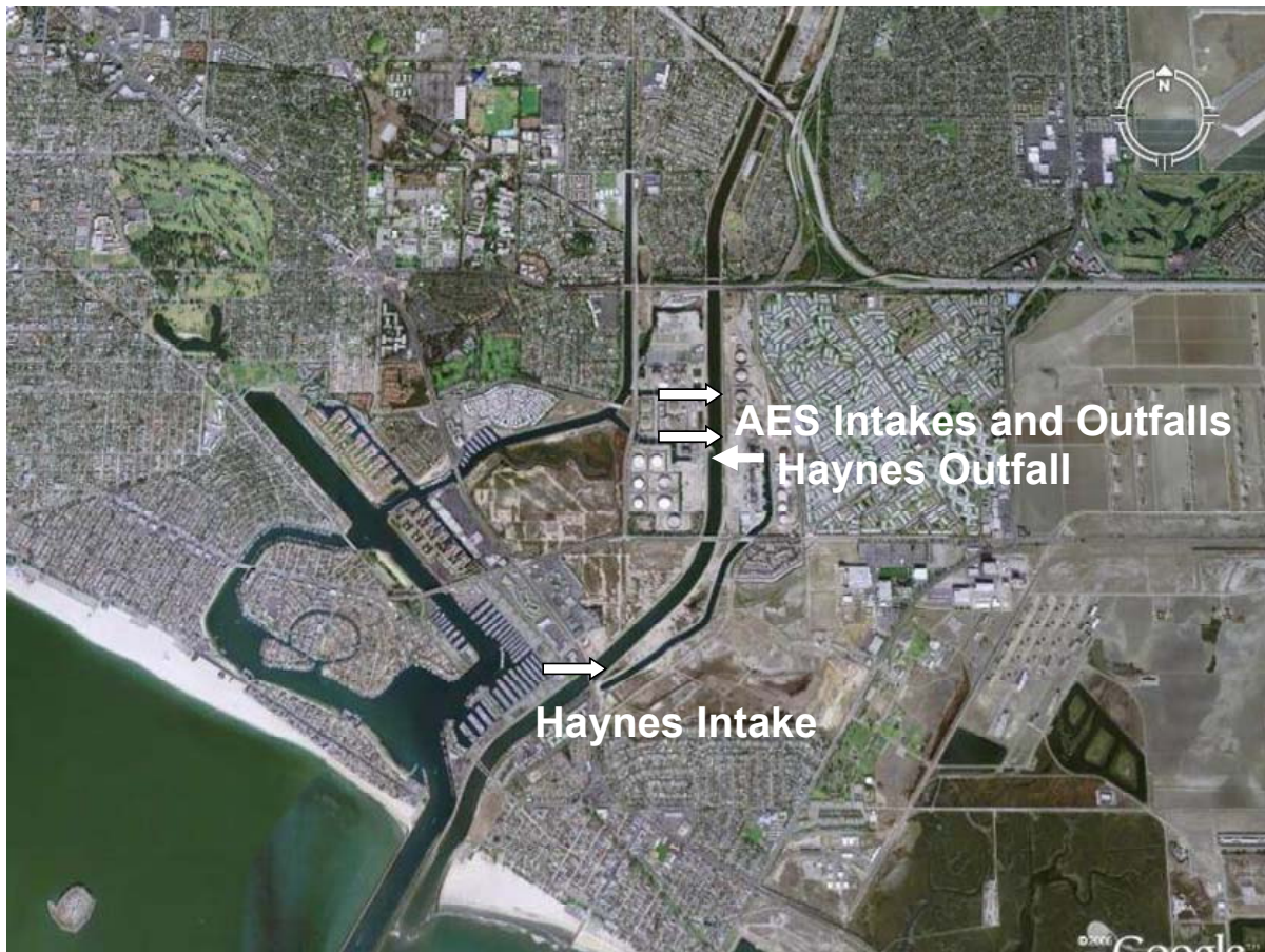
Figure 3-1 Power Plant Cooling Water Intake Locations
