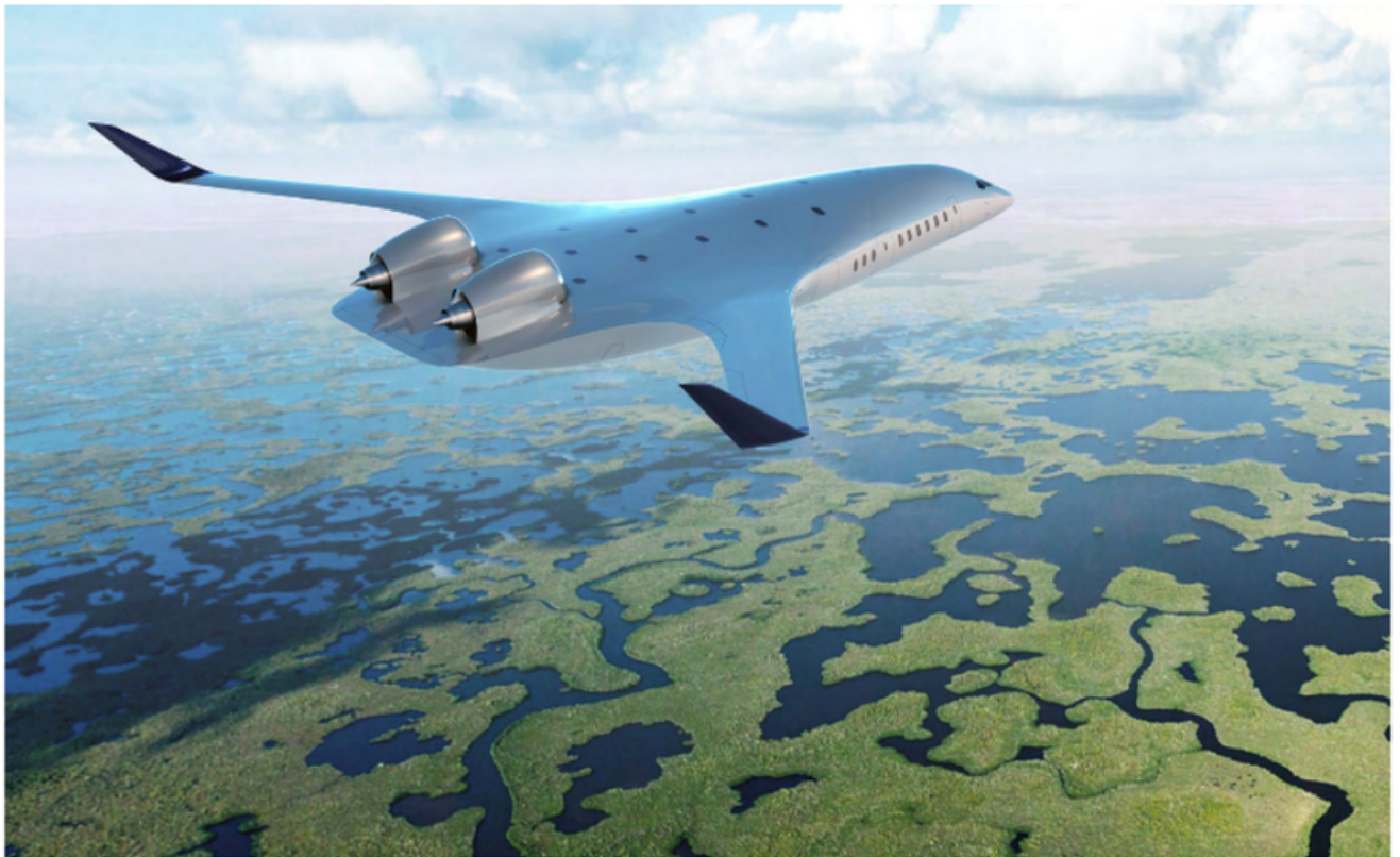
A rendering of JetZero's blended wing body Z5 aircraft. Courtesy of JetZero.
