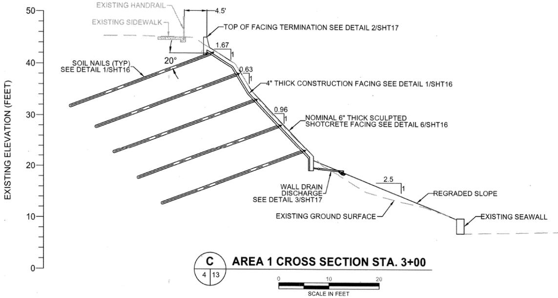
Figure 1 - Design Cross-Section of Soil Nailing
