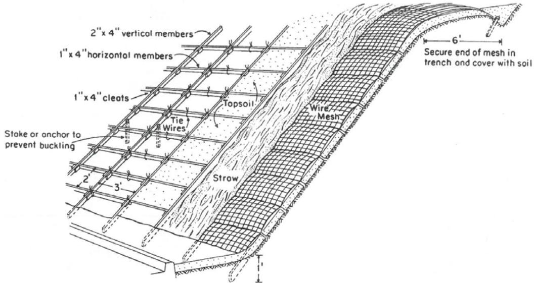
Figure 8-18. Anchored timber grid used to hold topsoil and slope plantings.
