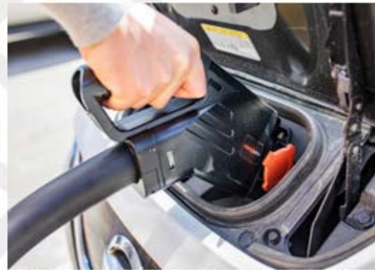
Nissan Leaf Plugging into a Level III Charger
